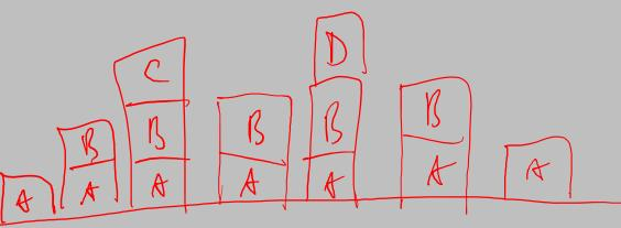
Simple and efficient implementation: Pointer separates allocated and freed space
