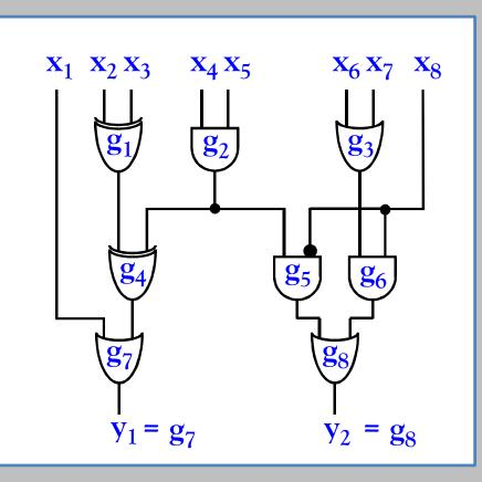
Types of gates:  $type(g_1) = type(g_4) = XOR_2$  $type(g_2) = type(g_6) = AND_2 \dots$
