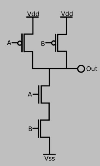
Output is 0 *iff* there is a transmitting path from 0 to the output, i.e., *iff* both n-type transistors transmit, a = b = 1, then NAND(a, b) = 0
